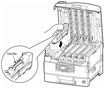
6. Push the lock lever as shown to lock the fuser in place.
